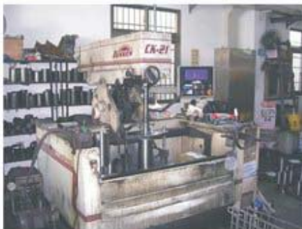
Computer Controlled /Vertical Axle Bore Semi-Finished Honing Machine. Bore Size Automatically Controlled,Honing Stone Automatically Compensation!!
