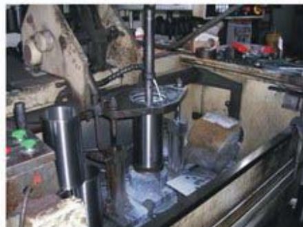
Computer Controlled /Vertical Axle Bore Semi-Finished Honing Machine. Bore Size Automatically Controlled,Honing Stone Automatically Compensation!!
